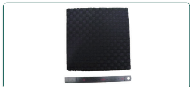
Fig.5 Our future study is MW-cured C-FRP composed of recycled carbon fiber and epoxy resin using vacuum assisted resin transfer molding method (VaRTM).
