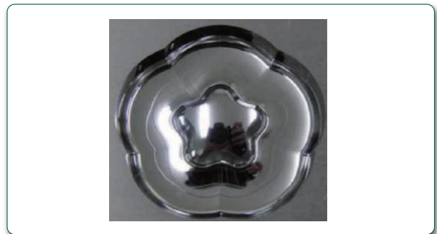
Fig.2 Mirror quality freeform surface of hardened steel machined by developed system
